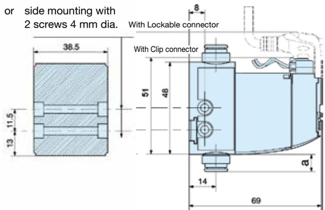
Dimensions and mountings of the stand-alone valves 4/2, double and single 3/2, 4/3 vented centre and 4/3 pressure centre.
