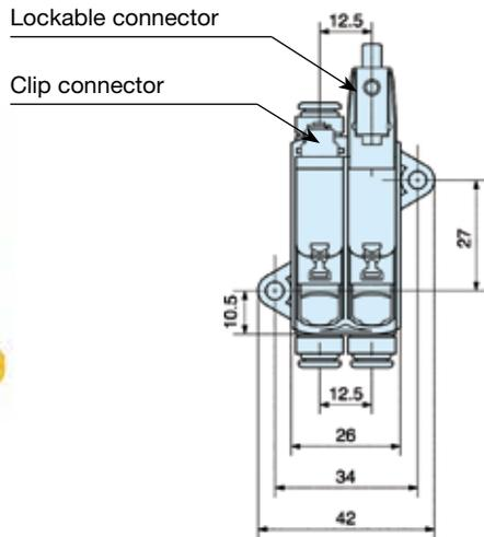
or side mounting with 2 screws 4 mm dia.
