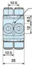
possible mounting with 2 screws 3 mm dia.
