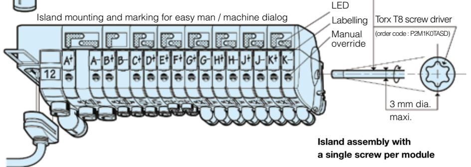
**Island assembly with a single screw per module**
