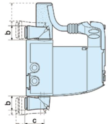
Reminder : peripheral modules may either be plugged in the valve output ports or mounted in line separate from the valve
