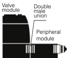
Stand alone valve complete with a plug-in peripheral module
