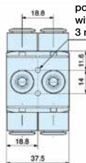
possible mounting with 2 screws 3 mm dia.
