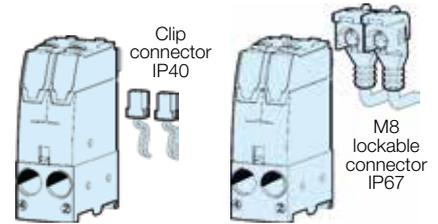
In its IP40 version, each solenoid shows Clip connection integrating LED and voltage surge protection. The clip connector with flying leads may be ordered separately with independent or interconnected common. In its IP67 version, each solenoid shows a M8 connection. Lockable connectors, IP67 protected, with LED voltage surge protection and flying lead cable may be ordered for the required length.
