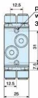
possible mounting with 2 screws 3 mm dia.
