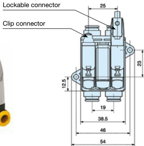
or side mounting with 2 screws 4 mm dia.
