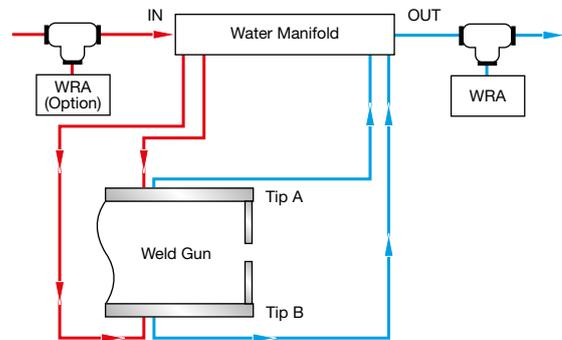
**Scenario 2**, the WRA can be placed on the **OUT** Line of the water manifold. In this situation, you would engage the unit and remove tip A first, replace it, and then remove tip B.
